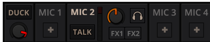
Fig. 1: The microphone ducking controls
