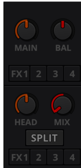
Fig. 20: The headphone and main mix knobs
