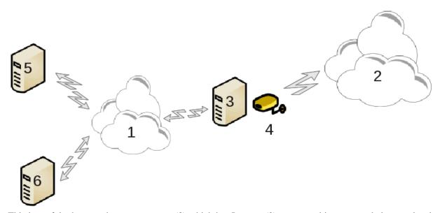
This is useful when you have a computer (3) which has Internet (2) access and is connected also to a local network (1). You can use computer (3) as a gateway to give that access to other workstations (5) and (6) in the local network (1). For this, the gateway must have two interfaces; the first one such as an ethernet card must be connected to the local network, and the second one (4) connected to the Internet (2).
