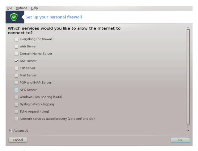
This tool<sup>44</sup> is found under the Security tab in the Mageia Control Center labelled "Set up your personal firewall". It is the same tool in the first tab of "Configure system security, permissions and audit".
