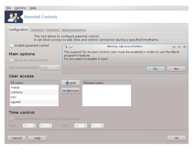
This tool<sup>46</sup> is found in the Mageia Control Center, under the Security tab, labelled Parental Control. If you don't see this label, you have to install the drakguard package (not installed by default).
