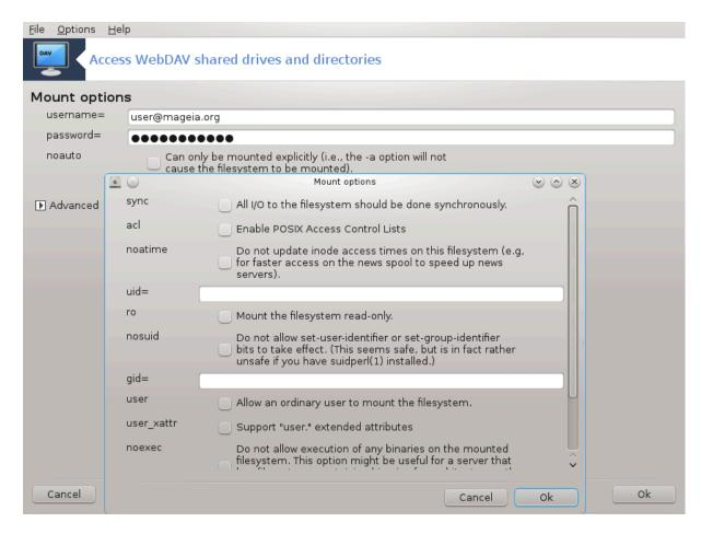
The option Mount allows you to mount immediately the access.
