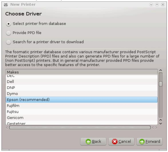
When you select a port, the system loads a driver list and displays a window to select a driver. The choice can be made through one of the following options.
