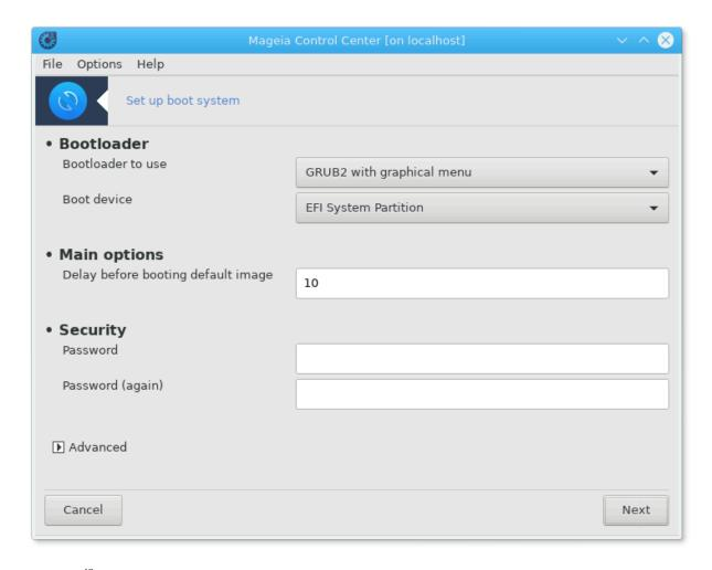
This tool<sup>48</sup> allows you to configure the boot options (choice of the bootloader, set a password, the default boot, etc.)
