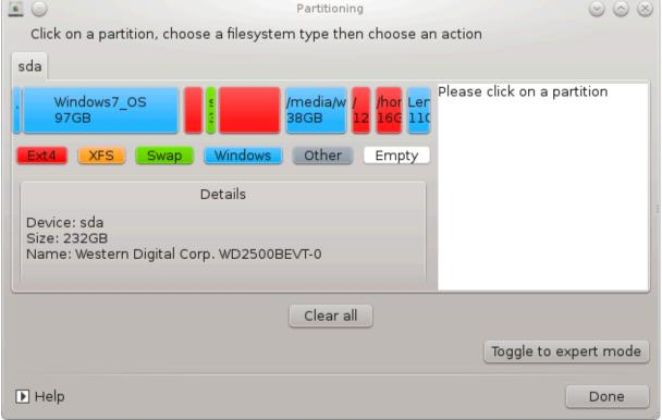
You can choose from many actions to adjust your hard disk to your preferences. Wiping an entire hard disk, splitting or merging partitions, resizing them or changing the filesystem, formatting or viewing what is in a partition: it is all possible. The Clear all button at the bottom is to erase the complete disk, the other buttons become visible on the right after you click on a partition.
